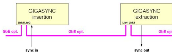
Figure 0 : Insertion and extraction of a synchronisation rythm on a Gigabit Ethernet link
